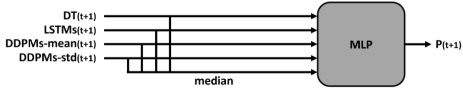
Figure 4: Architecture of the ensemble model included in the comparison
